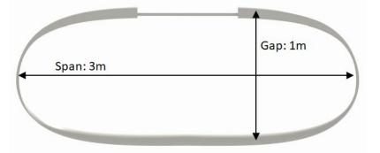
**Box Wing Specifications** Airfoil: Wortmann FX 63-137 Chord: 1 m (root), .55 m (tip)
