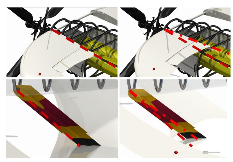
The two images on the left depict the wing and the strut that connects the bottom wing to the fuselage in their static position. The wing is pitched down 5° in the images to the right with the
