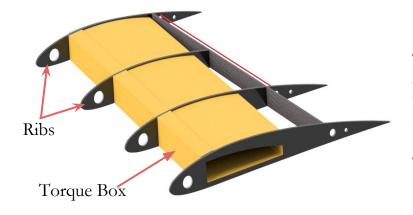
The internal structure of the fins consist of ribs and two angled spars that ensure a smooth transfer of the landing loads to the longerons.
